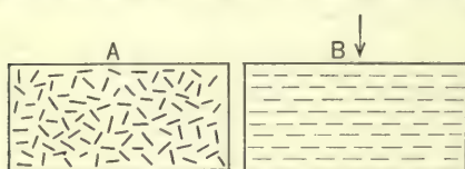
FIG. 41.—Diagram to illustrate the development of schistosity by pressure.
